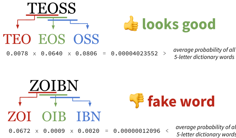
Figure 2: A visualization of how the Markov chain classifier works: by splitting the player’s submitted word into character trigrams, evaluating the likelihood of each trigram, multiplying together these likelihoods, and comparing to a probability threshold derived from actual English dictionary words of the same length.
