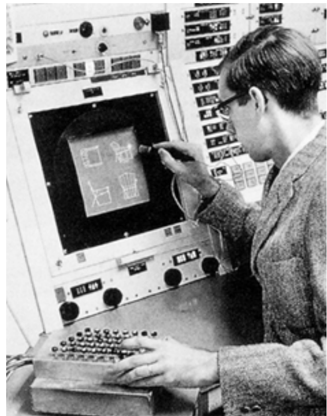
Figure-1: Ivan Sutherland’s SKETCHPAD. The user “sketches” on a 7 by 7 inch scope device with a 1024 by 1024 raster using a light pen and presses command buttons with the second hand
