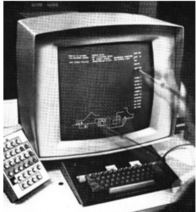
Figure-3: URBAN 5 ’s overlay and the IBM 2250 model 1 cathode ray-tube used for URBAN 5 .
