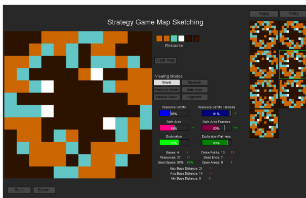
Fig. 2. Screenshot of the Sentient Sketchbook's interface. Alternative outputs are on the right, metrics and analysis are in the central area.
